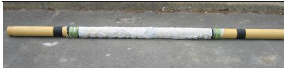
Figure 5. MPSP standpipe with barrier bag.
